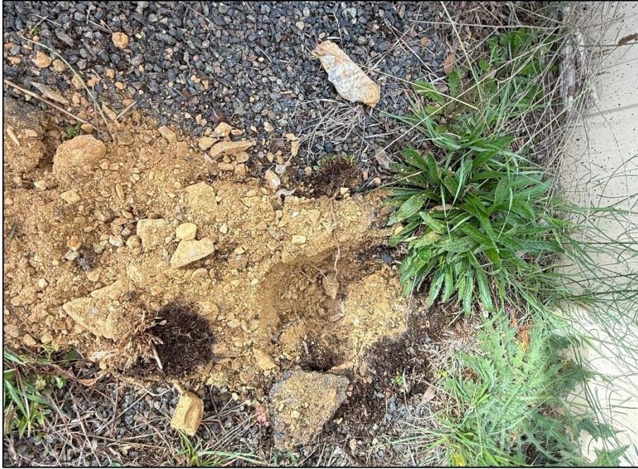
Plate 15: View of SS01 gravelly sand fill material located adjacent to the centre of the northern side of garage in the northeast portion of the Site. Dated 29 May 2025.
